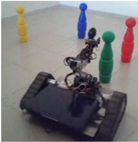
Fig. 5. Robot Kuzma-II. Design of this robot based on the well-known Johnny 5 Robot [53]. By utilizing heavy duty polypropylene and rubber tracks with durable ABS molded sprockets the robot has excellent traction. It includes two 12vdc 50:1 gear head motors and the Sabertooth 2 x 5 R/C motor controller. The electronic system based on SSC-32 microcontroller. Onboard computer of this robot is Asus Eee PC 1000HE. The robot is equipped with modified Lynxmotion robotic arm with wrist rotate and USB web camera Live! Cam Video IM Pro (VF0410).
