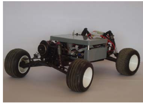
Fig. 3. Robot Kuzma-I. Design of this robot based on the well-known RC cars. From RC-CAR AT-10ES Thunder Tiger [50] we use only the four wheel chassis, the high torque DC-MOTOR and a steering servo. The DC-MOTOR drives the chassis and a steering servo controls the direction. The electronic system based on SSC-32 microcontroller. Onboard computer based on a motherboard with x86 compatible processor AMD Geode LX600 for embedded systems. The robot is equipped with USB web camera Live! Cam Video IM Pro (VF0410) [52].
