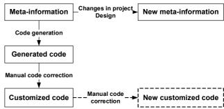
Fig. 2. The scheme of the automatic UI code generation for meta-information changing (the first alternative)
