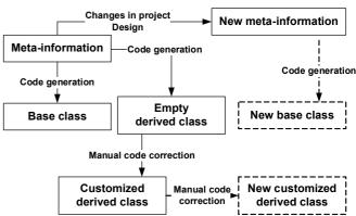
Fig. 6. The scheme of the hybrid approach of a UI for meta-information changing
